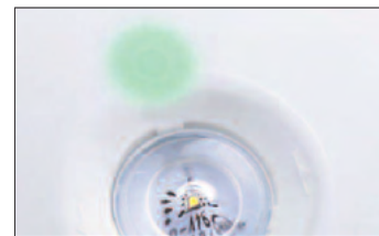
Operation indicator LED shines through a skin in housing plastic
