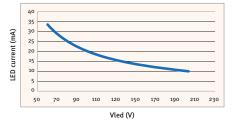
LDM200MO and LDM200MOD LED output current
