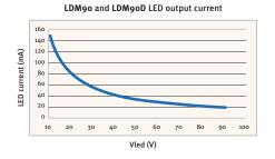
LDM90MO and LDM90MOD LED output current
