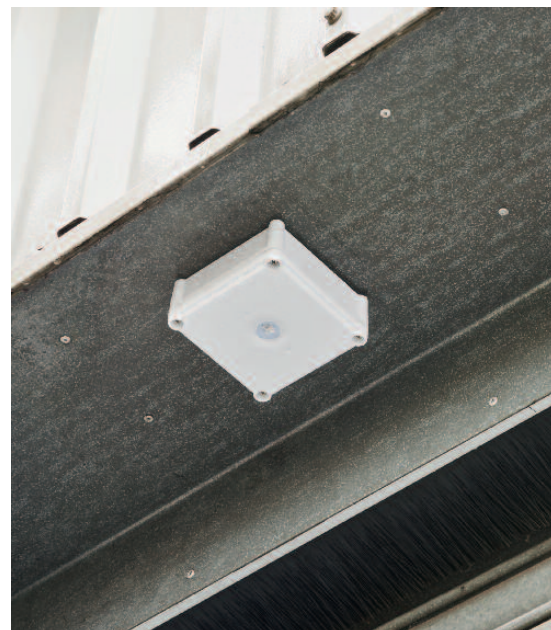
Operation indicator LED shines through a skin in housing plastic
