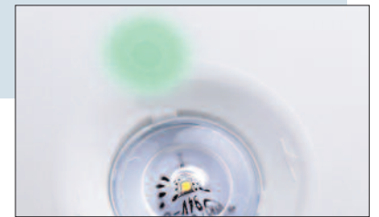
Operation indicator LED shines through a skin in housing plastic
